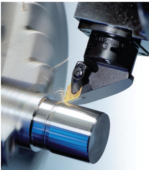
Fig. 1: A new generation of finish-turning tools keep close tolerances more consistently.
