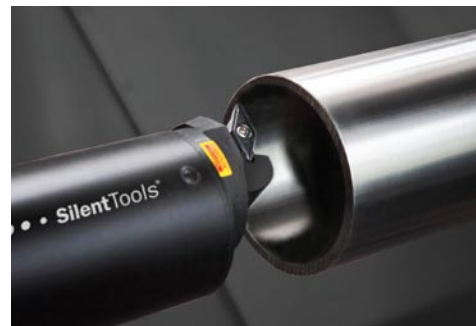
Fig. 5: Internal precision turning needs stable tool clamping and often vibration dampening.
