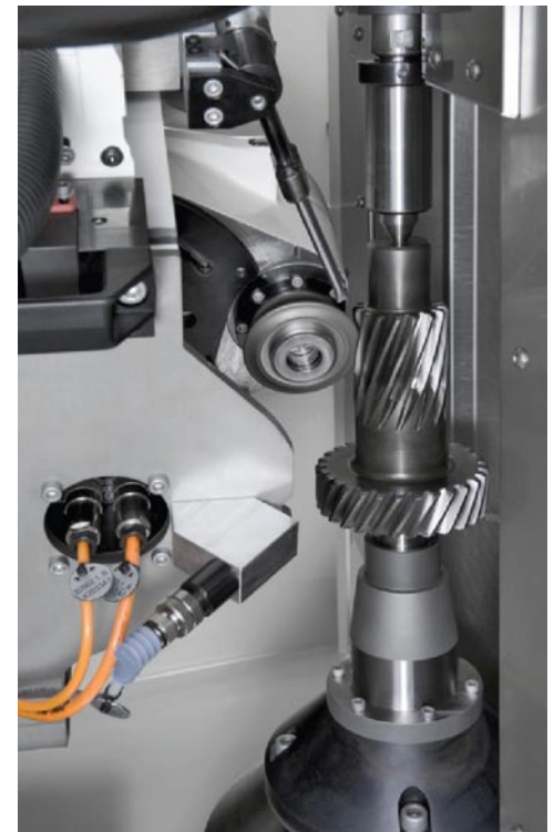
Fig. 3: Reishauer's new profile grinding spindle.
