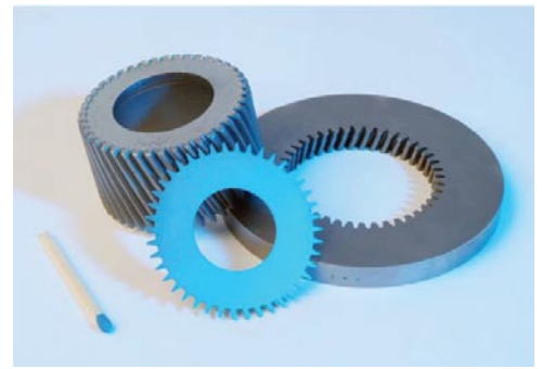
Fig. 2: A thin-plate electrode was used to machine an ID gear.
