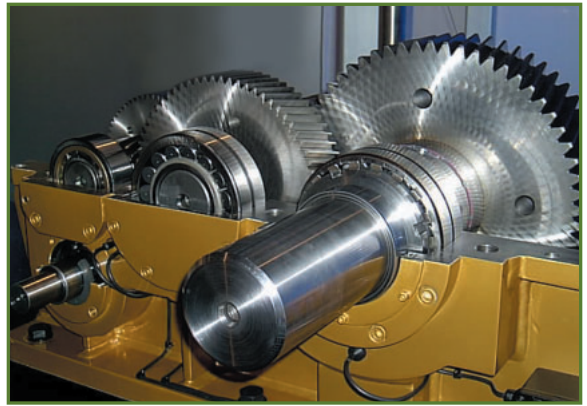
The 18k concept gearbox includes completely reengineered gears, which exceed most standard production quality levels. (Photo courtesy of SKF USA Inc.)
