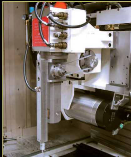
The NILES ZE 400 grinds both internal (shown here) and external gears in single and small-batch production. The machine also grinds parts from solids or pre-cuts.
