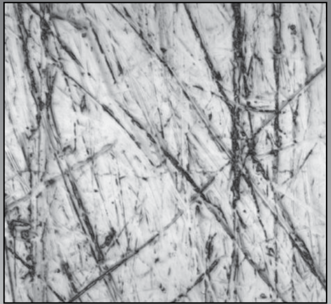
FIGURE 5: 2D EXTENDED DEPTH OF FOCUS IMAGE OF CUT MIKRONITE PART SURFACE GENERATED USING ZEISS CONFOCAL LASER SCANNING MICROSCOPE WITH 100X/0.95 OBJECTIVE LENS AND 543NM LASER WAVELENGTH.
