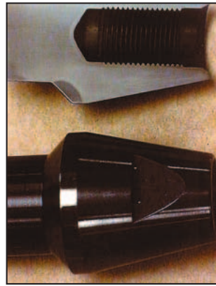
Figure 4 — Specialty valve laser heat treated to a controlled depth. Treated without overlap by moving laser beam at high speed.
