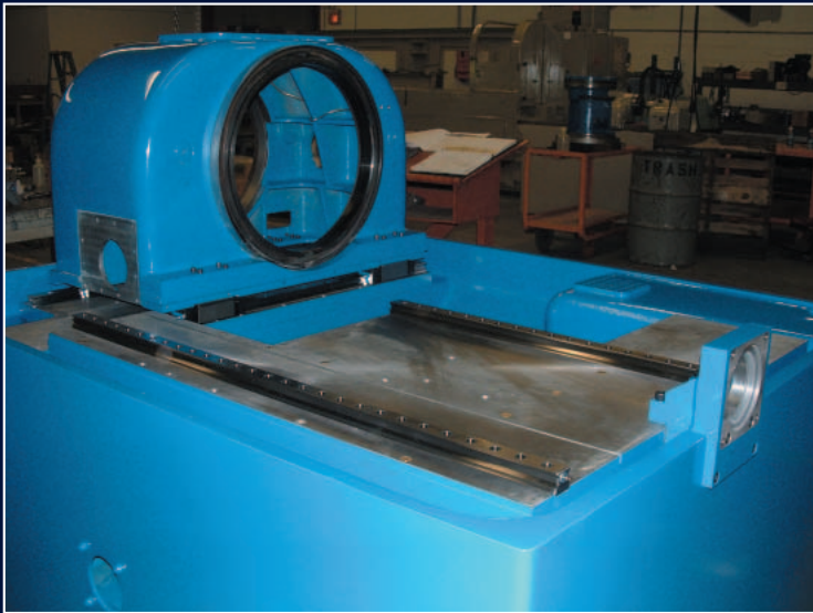
Linear ways provide high stiffness, long life and ease of repair
