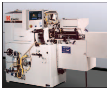
Figure 8 — Cylindrical die worm rolling machine with automatic shaft feeder
