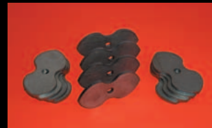
Figure 2 — Photograph of epitrochoidal spur gears such as shown in Figure 1 for R=2:1 speed ratio.
