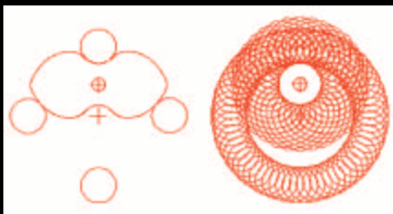
Figure 1 — Two-tooth partially conjugate prolate epitrochoid spur gear reducer of parallel input/output shafts for ratio R=2:1 .
