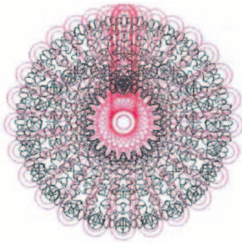
Figure 4 — Full-turn epicycloid (cardioid) indexer using two identical involute spur gears.
