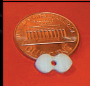
Figure 3 — Miniature version of the gears shown in Figure 2. Reduced in size to a scale of 1:16 (6.25 percent) approximately, this gear was precision cut in acetal, an engineering thermoplastic.
