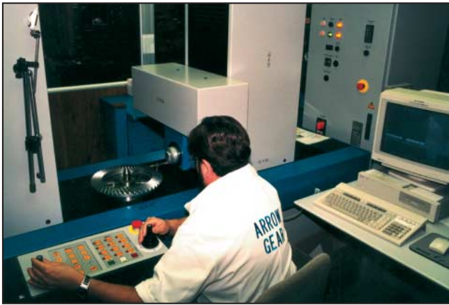
The Zeiss/Höfler CNC Gear Inspection System is used in conjunction with Arrow's Computer Controlled Manufacturing (CCM) Closed Loop System for the inspection of spiral and hypoid bevel gears during tooth cutting and grinding operations.
