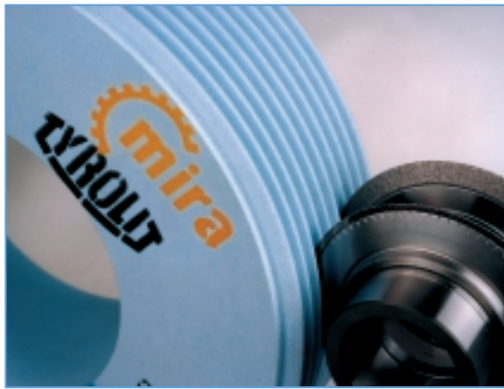
◀ Figure 1: MIRA multi-ribbed grinding tool (sintered aluminum oxide with micro-structure in vitrified bond) with dressing wheel set (diamond, electroplated).
