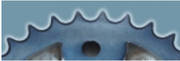
Powder Metal Sprocket heated with Simultaneous Dual Frequency (SDF). 160 kW MF-Power (12 kHz) and 80 kW HF-Power (250 kHz) for 0.2 seconds. Note perfect contouring with the part with no through hardening of the teeth. Uniform hardness depth of 1.0 mm to 1.2 mm at HRa 74 mass quenched. Sprocket is 100 mm in diameter with 32 teeth. Tooth thickness is 5.2 mm.
