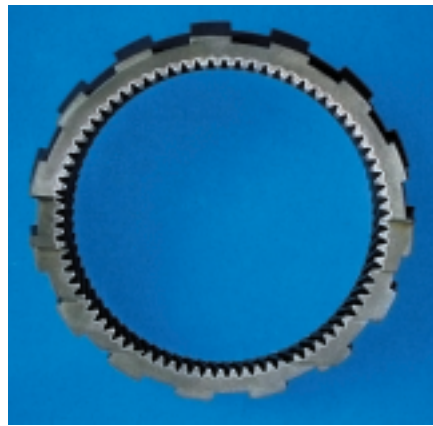
Ring Gear. Heat Time 0.49 Sec. SDF 400kW MF / 200 kW HF
