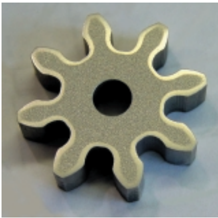
Gear. Heat Time 0.19 Sec. SDF 135 kW MF / 47 kW HF
