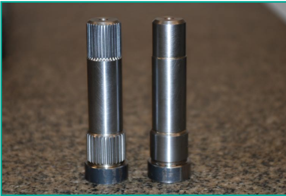
Figure 2: Blank and finished output shaft with two rolled splines.
