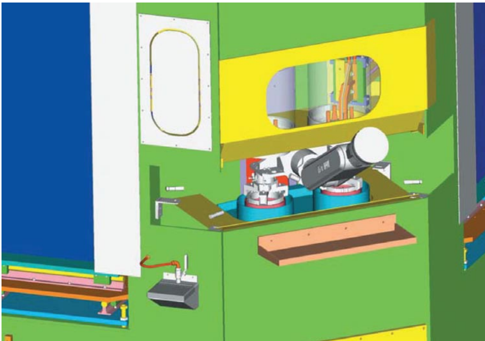
Robotic load operation mechanism for SPF induction hardening in-line integration.
