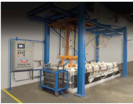
Fig. 3: Gears and similar power transmission components like these can be blackened, assembled, and shipped to order same day with an in-house low temperature black oxide system.
