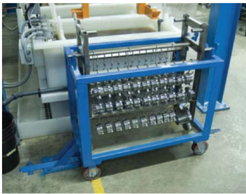
Fig. 5: Carts carry unfinished parts to the CNC process line where an automated hoist takes over, moving the rack through the finishing tanks with accurate timing.
