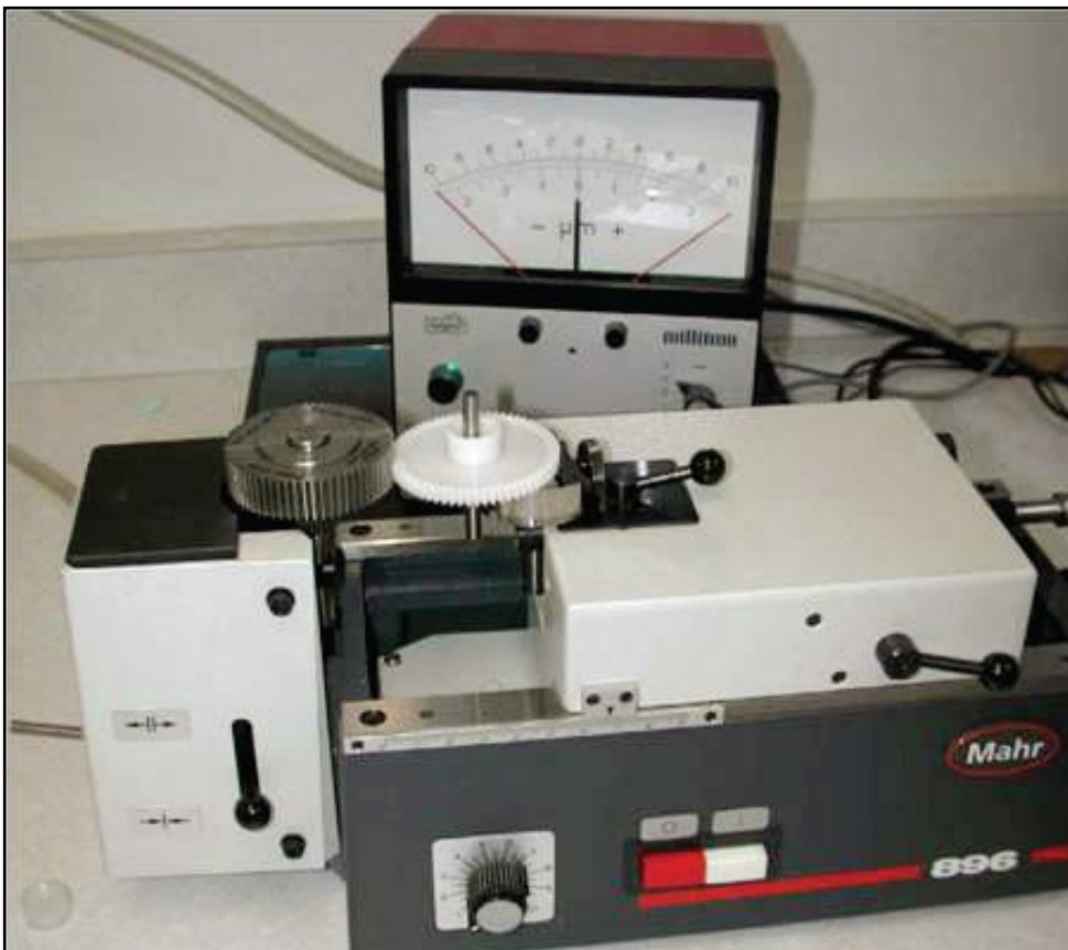
FIGURE 3: CNC ROLL TESTER ADAPTED FROM MAHR
