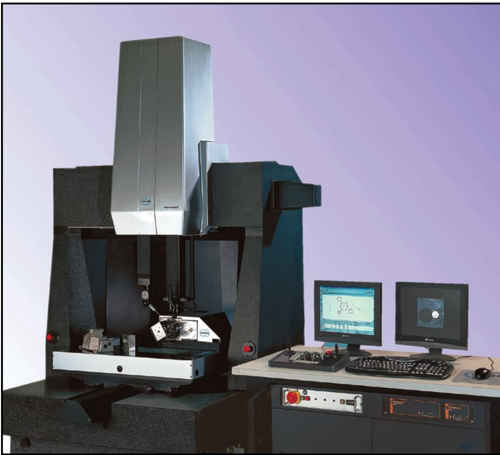
FIGURE 1: WERTH IP/VIDEO VHECK (CMM) SUPPLEMENTED WITH KLEISS POLYMER ANALIZATION SOFTWARE
