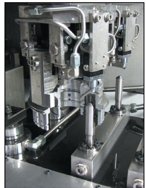
Fig. 5: Internal part feature being deburred. Cross section illustrates how internal features are reached.
