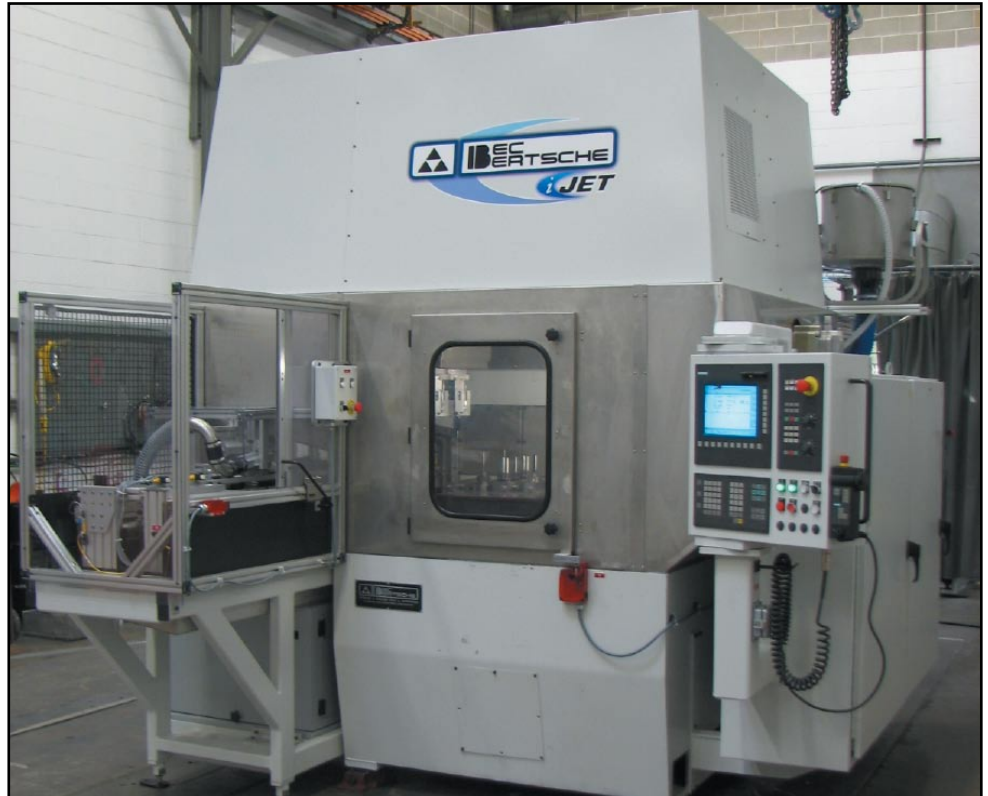
Fig. 3: Bertsche 4-axis (X, Y, Z, and C axis) i-Jet with integral drying station and post deburr/part rinse station.
