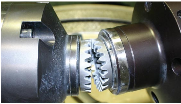
Fig. 2: Typical straight bevel gear contact pattern.
