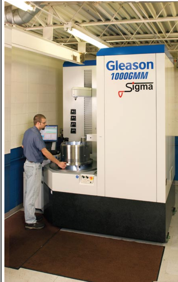
Fig. 3: Schafer Gear Works' new 1000GMM analytical gear inspection system can accommodate gears as large as 1000mm in diameter and 1300mm in length.
