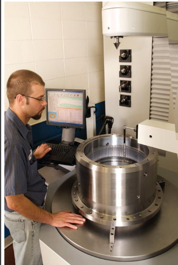
Fig. 4: Using Gleason’s GAMA software, Schafer operators can check important characteristics such as lead, index, and profile in half the time on this large 109-tooth, internal spur gear. Note the use of a Renishaw SP80H 3-D scanning probe, with various stylus sizes and configurations, interchangeable from an automatic probe changer.
