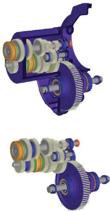
Fig. 6: A five-speed transaxle gearbox
