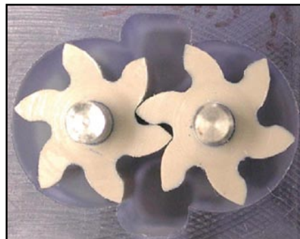
FIG. 13: THIS MEDICAL PUMP DEMONSTRATES THE DIRECTLY DESIGNED FLEXIBLE ASYMMETRIC TEETH THAT PROVIDE A BETTER SEAL BETWEEN THE GEARS AND THE HOUSING, RESULTING IN HIGHER OUTPUT PRESSURE, FLOW, AND EFFICIENCY.
