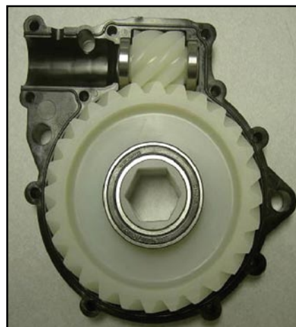
FIG. 12: THESE CROSSED HELICAL GEARS ARE USED IN AGRICULTURAL EQUIPMENT. IT WAS POSSIBLE TO REPLACE AN OLD-STYLE METAL CHAIN DRIVE WITH A LESS EXPENSIVE, SAFE, AND MAINTENANCE-FREE PLASTIC GEAR DRIVE AND FLEXIBLE SHAFT.
