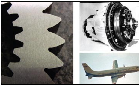
FIG. 15: THE TWO-STAGE PLANETARY GEAR REDUCER OF THE TURBO-PROP ENGINE TV7-117 (DESIGN BUREAU NAMED AFTER V.Y. KLIMOV, ST. PETERSBURG, RUSSIA) FOR THE TWO-ENGINE ILYUSHIN-114 PLANE (CURRENTLY IN PRODUCTION) HAS ALL GEARS WITH ASYMMETRIC TEETH. APPLICATION OF THE ASYMMETRIC TEETH HELPED TO PROVIDE VERY LOW WEIGHT TO OUTPUT TORQUE RATIO AND CUT DOWN DURATION AND EXPENSE OF OPERATIONAL DEVELOPMENT.
