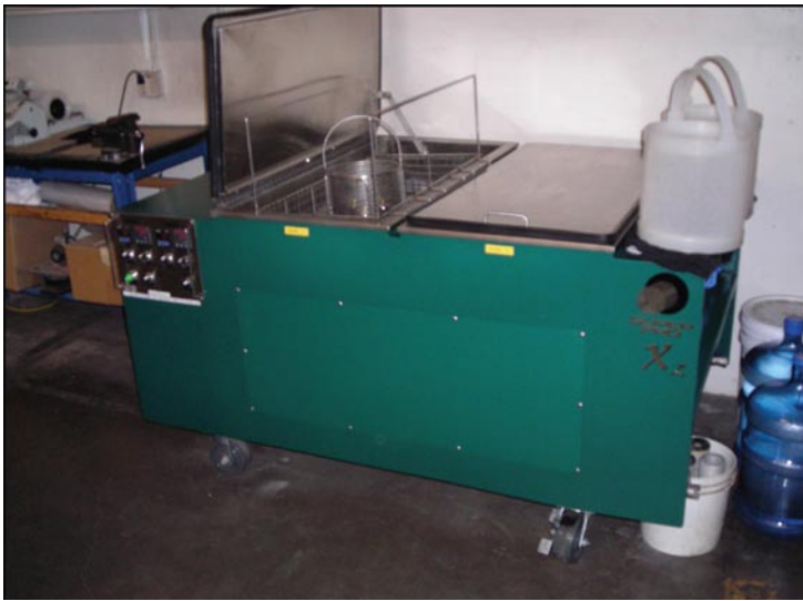
Fig. 3: The ultrasonic cleaning tank generates millions of microscopic bubbles per second, cleaning even the hardest to reach areas.
