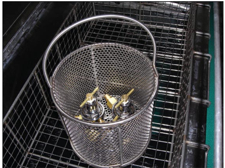
Fig. 2: Parts can simply be placed in a tank of environmentally friendly, water-based cleaning soap and the switch flipped for the cleaning process to begin.
