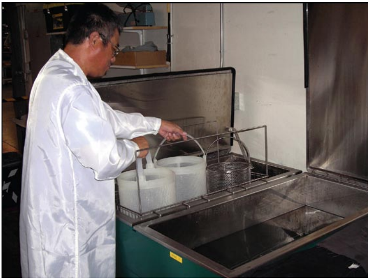
Fig. 1: Ultrasonic parts cleaning is commonly used to streamline a variety of manufacturing and maintenance processes.
