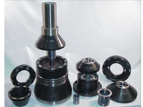
Fig. 2: Universal base fixture, interchangeable between multiple machines
