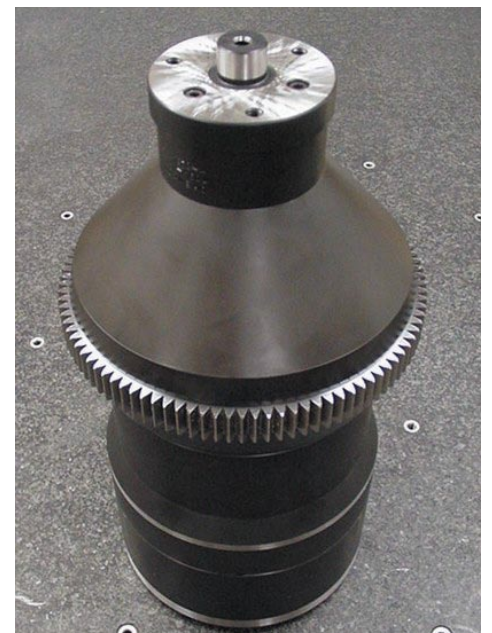
Fig. 4: Dry hob rigid tooling
