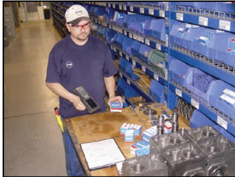
PROPER HANDLING MANDATES LEAVING BEARINGS, GEARS AND SEALS IN THEIR BOX UNTIL THEY ARE READY FOR INSTALLATION.
