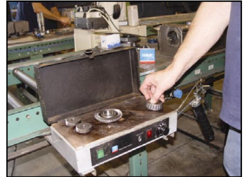
HEATING A BEARING, WHICH EXPANDS THE INNER RACE FOR FITTING ONTO ITS ASSIGNED SHAFT, IS BEST ACHIEVED WITH AN INDUCTION HEATER OR A HOT PLATE.
